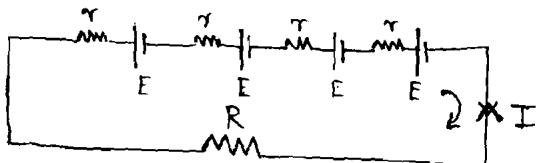
The four cells are shown in the diagram. We now consider the potential over the whole circuit.
